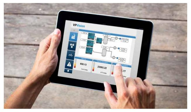
In the P&ID module you can place real time widgets on a background diagram.
